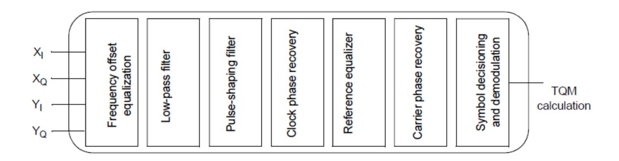
The basic blocks that are required for a reference receiver implementation are illustrated
