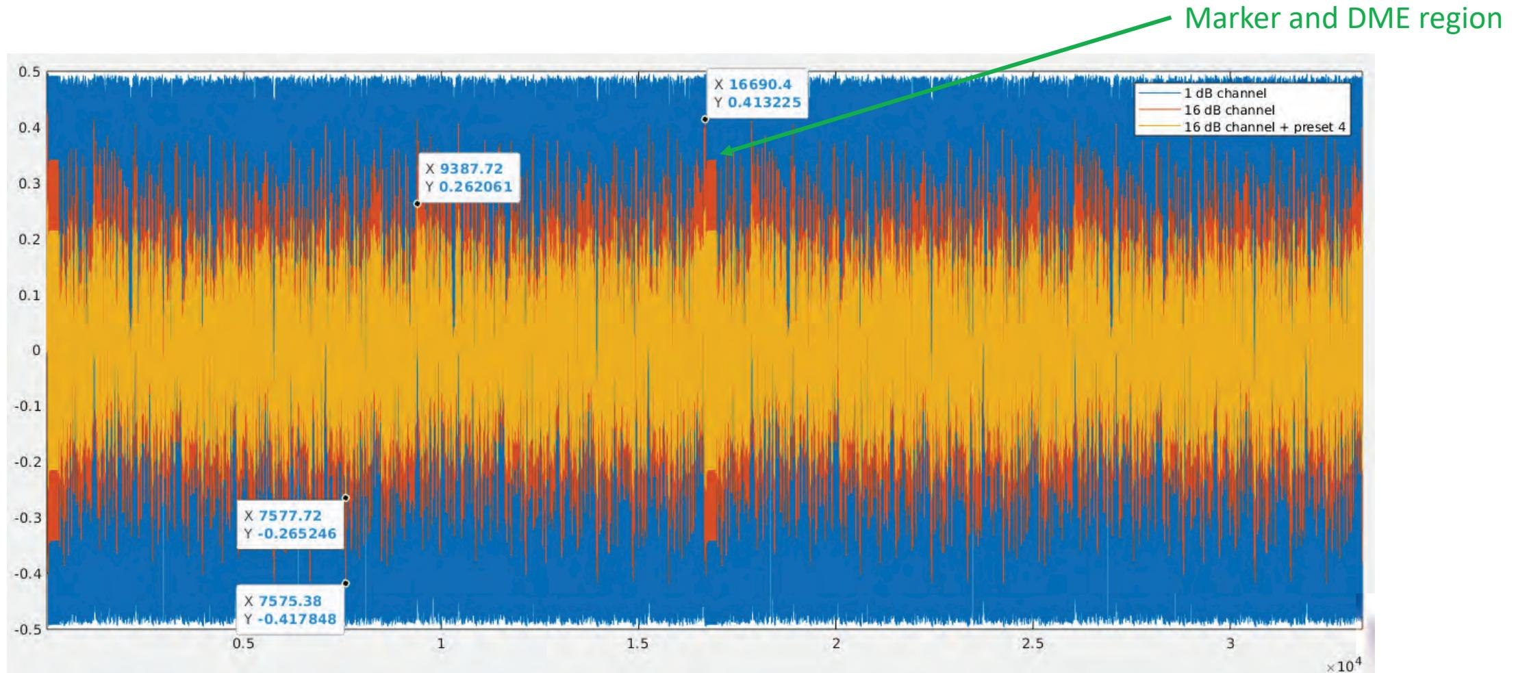
The signal is attenuated by the channel and by the Tx equalizer – the Tx output swing is never seen by the receiver
