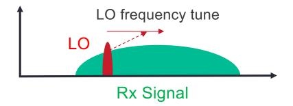
A locked LO laser with ~± 4 GHz tuning range will not guarantee interop with less accurate lasers
