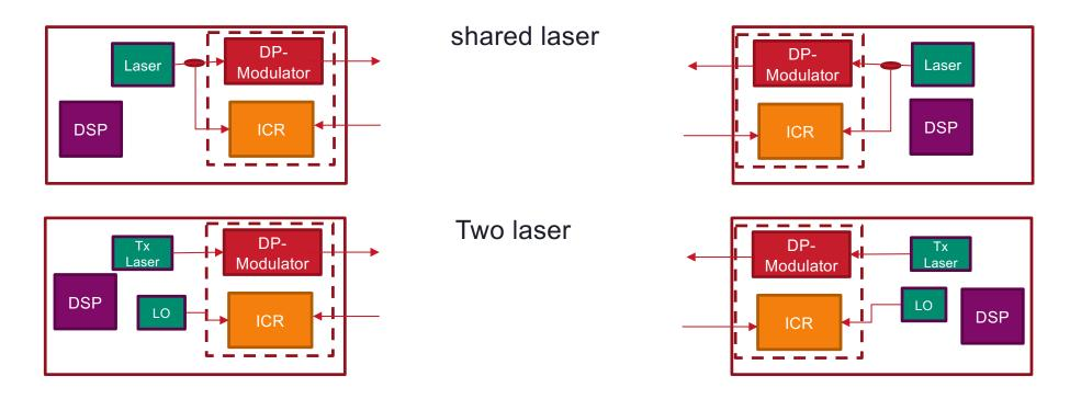
Typical coherent implementation uses a shared laser for both Tx & Rx (LO)
