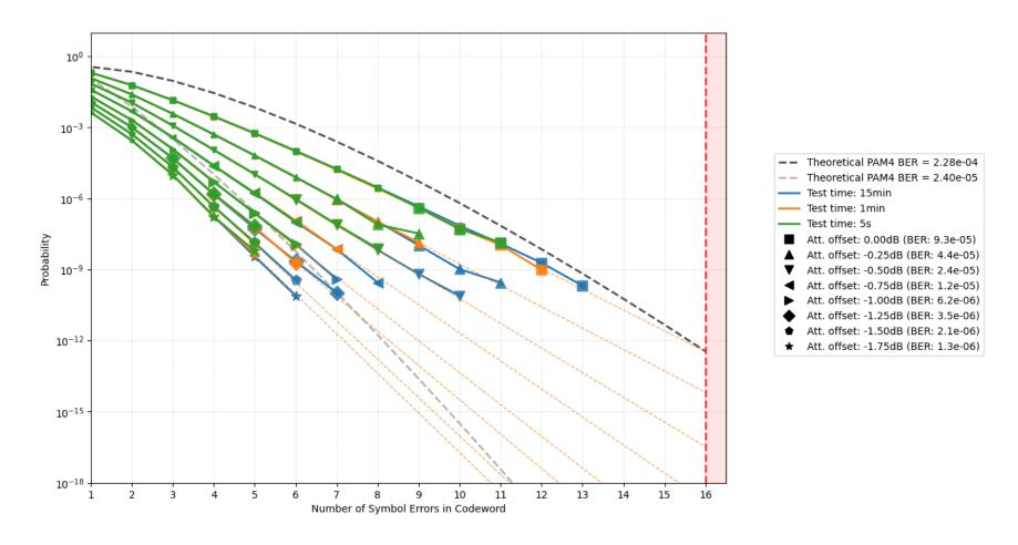
With attenuation set to the Rx sensitivity limit, the 1.5 dB functional\_test\_margin crosses the Functional Mask around 1e-18 probability.
