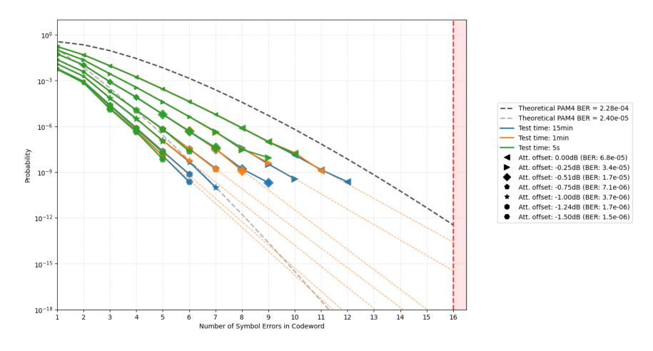
Although this transmitter had some Tx OMA margin, it still crosses the functional mask before reaching a probability of 1e-18, even with a 1.5 dB functional\_test\_margin applied.
