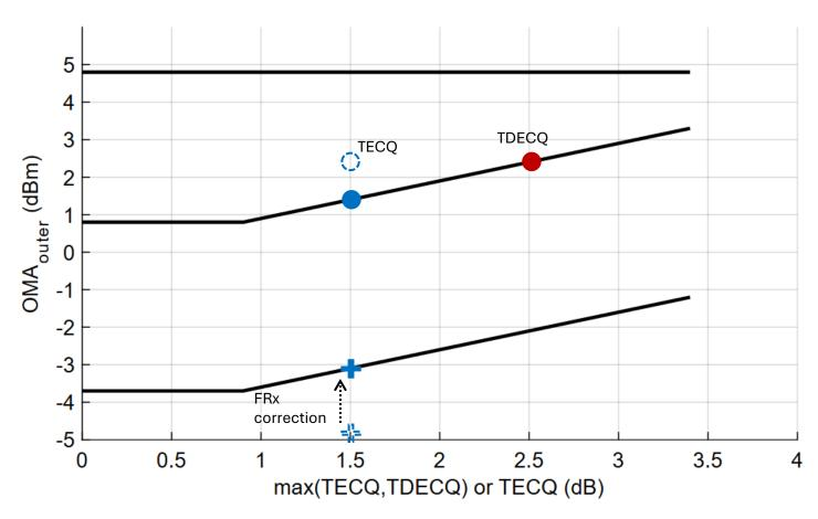
Adjust FRx sensitivity (based on block error ratio) upward by its margin to align with the spec limit.
