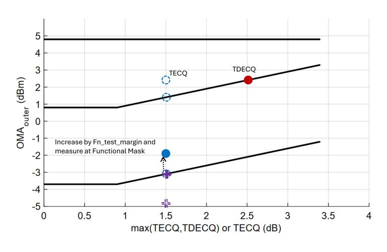
Increase receive input power into FRx to test closer to the typical operating point instead of at the SNR limit
