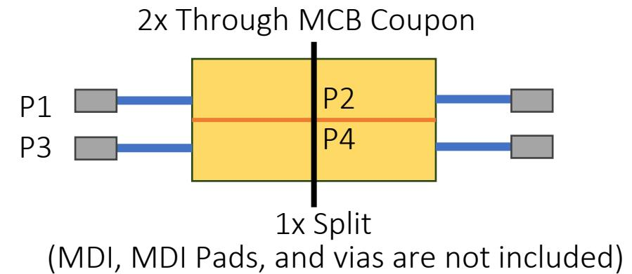
The 1x through characterization file is extracted from a 2x through MCB coupon measurement. It is not extracted from the exact MCB in the MTF measurement, but it is a representation of it.
