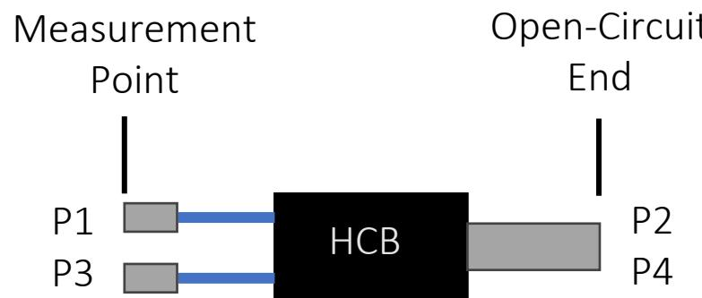
The 1x through characterization files are extracted from the exact HCB used in the mated measurement. 1x throughs are generated from the open-circuit measurement of each differential pair. The edge card fingers are included.
