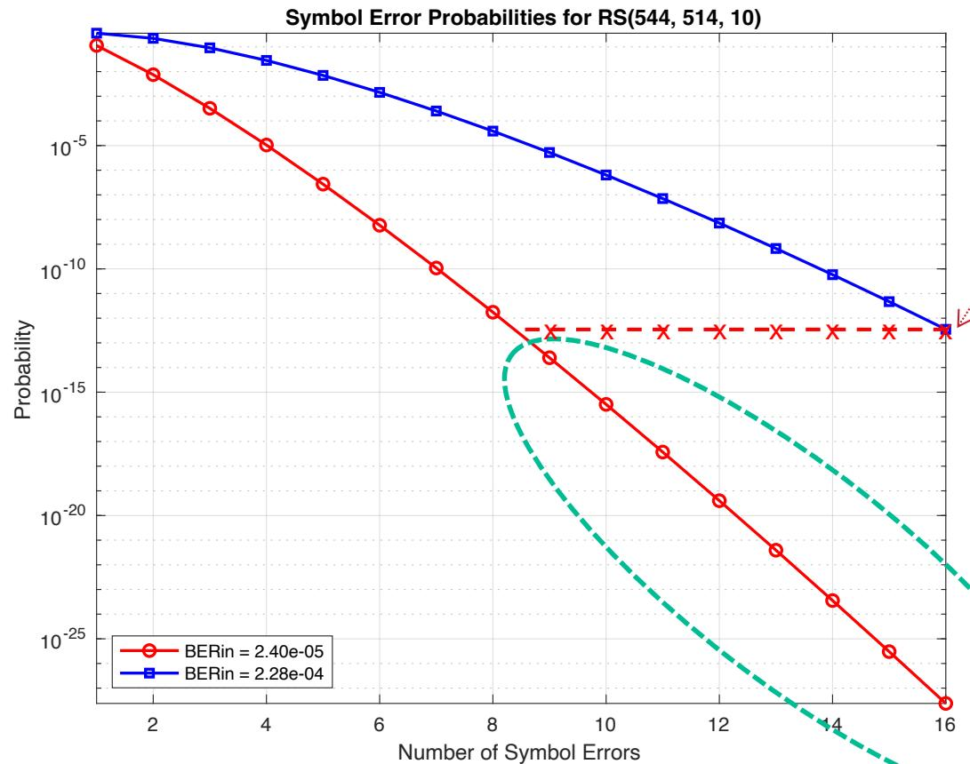
To deal with low probability values the Transmitter functional symbol error mask (Table 180-18) values for > 8 Symbol errors were replaced with a value corresponding to 16 symbol errors/codeword for a 2.28e-4 BER in D2.2.
