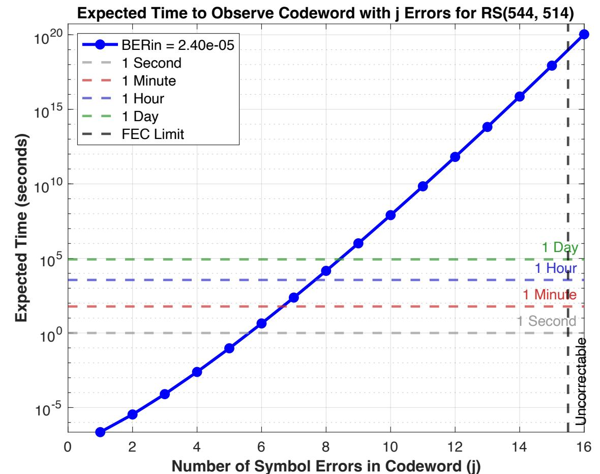
Note: If an RS FEC decoder is used to measure the symbol errors, 16 is likely not available
