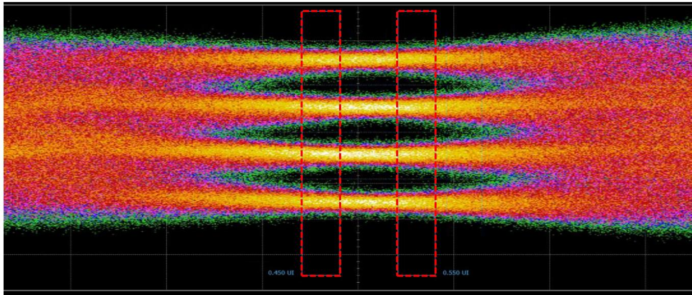
**TDECQ** builds a single distribution from samples across all symbols of the entire SSPRQ pattern, making it a consistent distribution that is largely insensitive to the scope random sampling phase and noise of a particular measurement instance.
