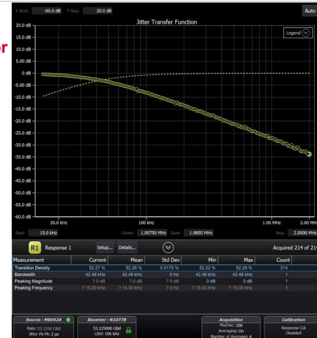
P8023dj: Jitter Transfer Function (JTF) analysis 11/2024
