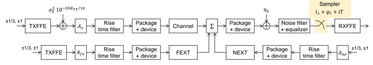
Given the peak Dual-Dirac jitter  $A_{DD}$ , the RMS random jitter  $\sigma_{RJ}$ , and  $h_J(i)$  which is the slope of victim signal path pulse response around the sampled values ...
