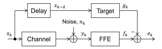
Equivalent model when slicer outputs are correct i.e.,  $\hat{x}_k = x_{k-d}$
