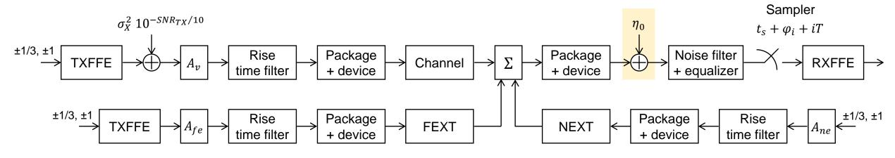
Given the transfer function of the receiver noise filter  $H_r(f)$ , the transfer function of the continuous-time equalizer  $H_{ctf}(f)$ , and one-sided power spectral density  $\eta_0$  (converted to units V<sup>2</sup>/Hz) ...
