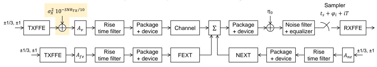
Given the transmitter signal-to-noise ratio  $SNR_{TX}$ , the transfer function of the rise time filter  $H_t(f)$ , and the voltage transfer function of the victim signal path  $H_{21}^{(0)}(f)$ , ...
