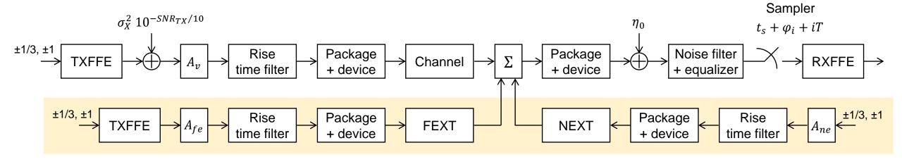
Given the signal power  $\sigma_X^2 = \frac{L^2 - 1}{3(L - 1)^2}$  where L is the number of signal levels and ...
