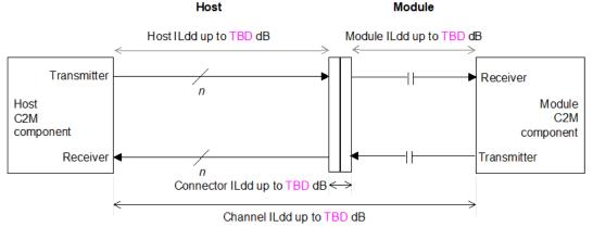
NOTE—The number of lanes *n* is equal to 1 for 200GAUI-1, 2 for 400GAUI-2, 4 for 800GAUI-4, and 8 for 1.6TAUI-8. ILdd values are at 53.125 GHz.
