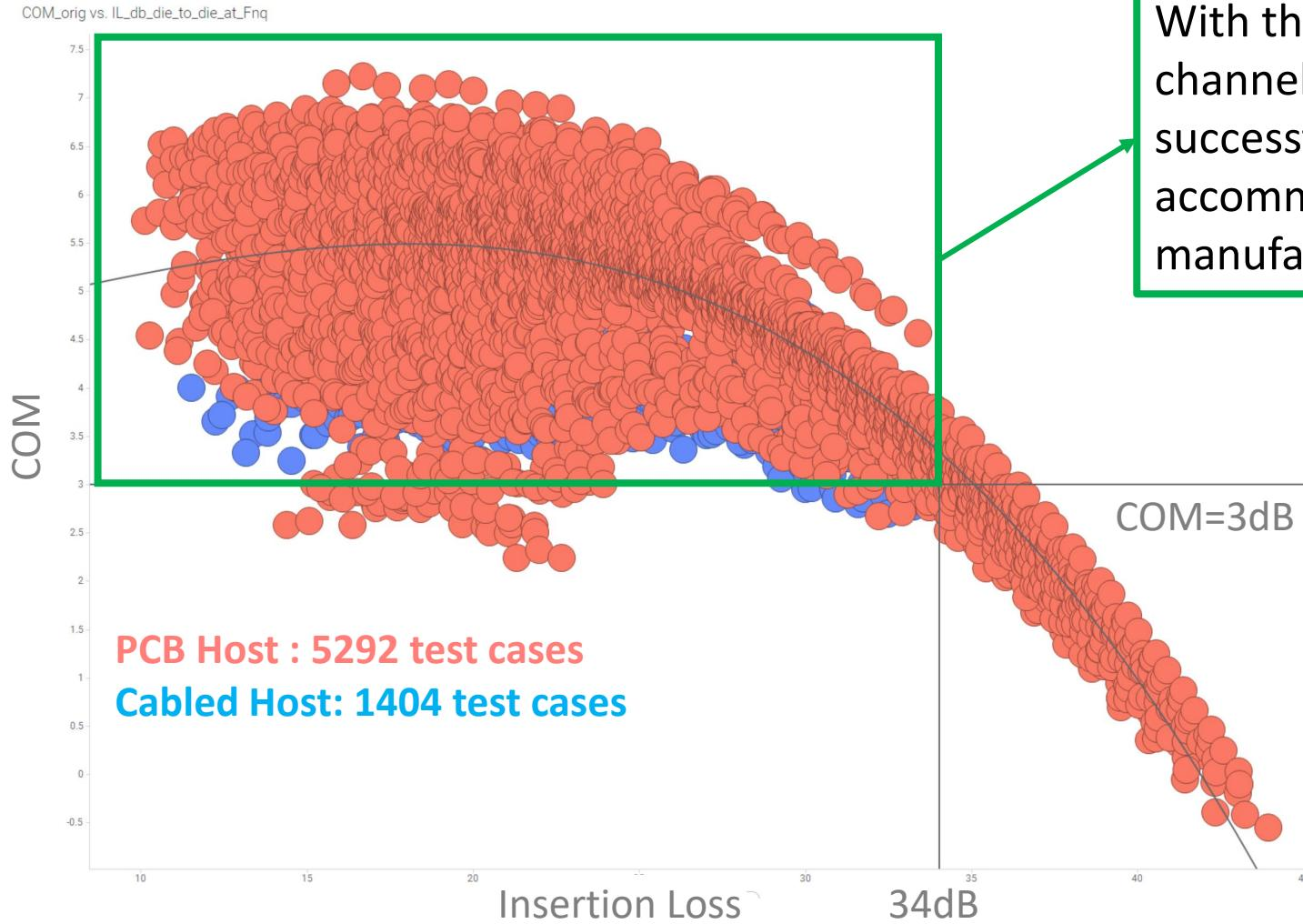
With the adopted reference RX, most channels within the loss target successfully pass 3 dB COM, accommodating both implementation and manufacturing variations.
