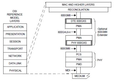
800GAUI-n = 800 Gb/s n-LANE ATTACHMENT UNIT INTERFACE 800GMII = 800 Gb/s MEDIA INDEPENDENT INTERFACE 800GXS = 800GMII EXTENDER SUBLAYER DTE = DATA TERMINAL EQUIPMENT MAC = MEDIA ACCESS CONTROI MDI = MEDIUM DEPENDENT INTERFACE PCS = PHYSICAL CODING SUBLAYER PHY = PHYSICAL LAYER DEVICE PMA = PHYSICAL MEDIUM ATTACHMENT PMD = PHYSICAL MEDIUM DEPENDENT
