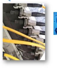
Contaminated fiber connectors commonly seen at both optical module and ODF:
