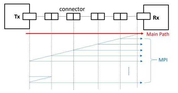
For multiple reflections in the link, the received optical signal is (assume cw signal transmitted):
