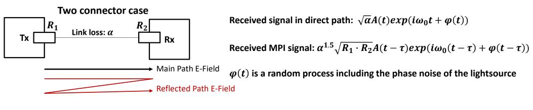
$$I(t) = |mainPath + reflectedPath|^{2} = \alpha A(t)^{2} + \frac{2\alpha^{2}\sqrt{R_{1} \cdot R_{2}}A(t)^{2}\Re(exp(i\omega_{0}\tau + \varphi(t) - \varphi(t - \tau)))}{\text{Multipath interference}} + \frac{\alpha^{3}R_{1}R_{2}A(t)^{2}}{\text{Very small, negligible}}$$
