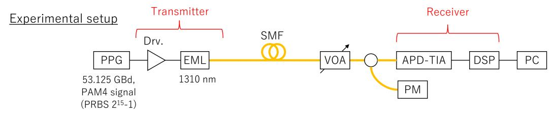
PPG: pulse pattern generator, Drv.: driver, EML: external modulated laser, SMF: single mode fiber, VOA: variable optical attenuator, PM: power meter, TIA: trans impedance amplifier, DSP: digital signal processing
