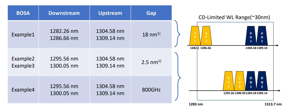
This wavelength plan example takes into account the LWMD wavelength and allows for flexible adjustments within the CD-limited WL range.
