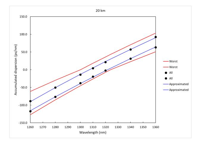
1294 nm min CD = -51.5 ps/nm 1310 nm max CD = 6.7 ps/nm
