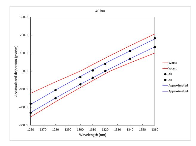
1294 nm min CD = -97 ps/nm 1310 nm max CD = 6.3 ps/nm
