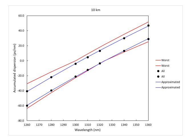
1294 nm min CD = -26.8 ps/nm 1310 nm max CD = 4.4 ps/nm
