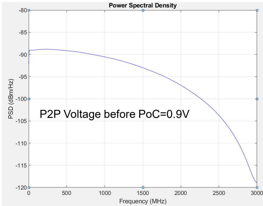
PSD shown with normal mode signal level but with continuous transmission, no quiet gap.
