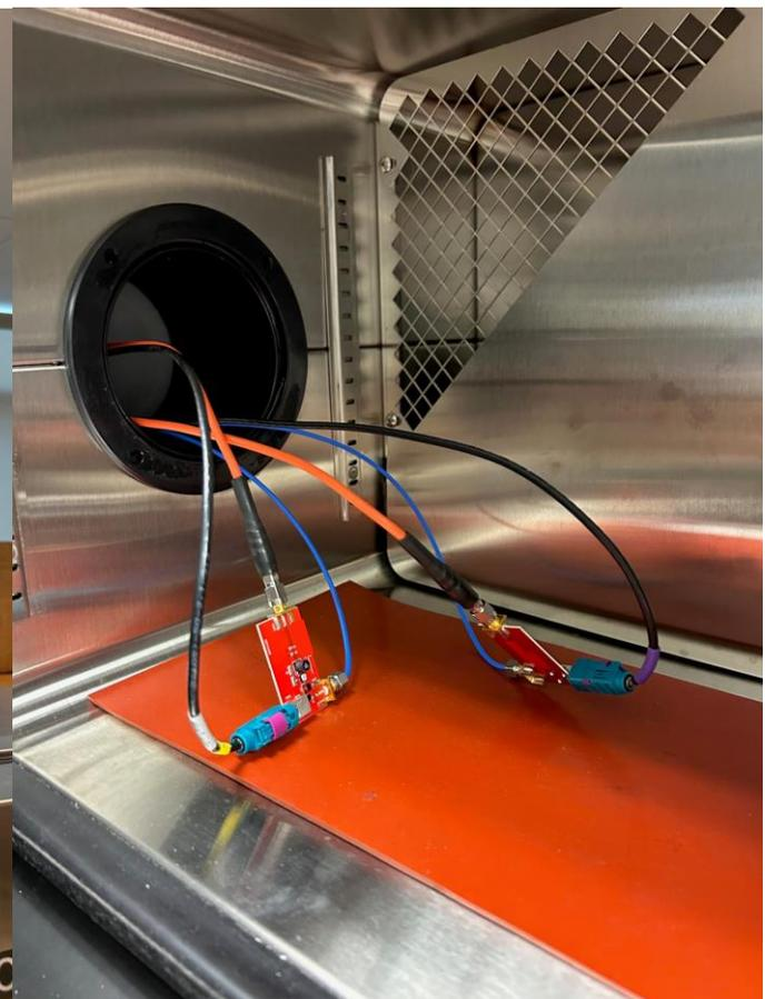
PoC coupon boards inside oven chamber
