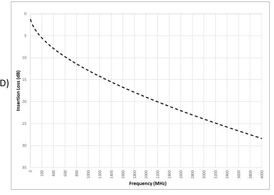
The insertion loss is illustrated in Figure 2xx-TBD. The requirements are to be based on the data rate and modulation. For the 2.5 Gb/s PAM2 the requirements are applicable to 2.0 GHz. For the 5.0 Gb/s PAM2 and the 10 Gb/s PAM 4 the requirements are applicable to 4 GHz.
