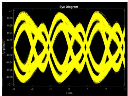
Waveform after S&H MF, assuming clock is recovered, and it is at the best sampling phase.
