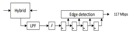
Missing blocks: HPF, RX Clk Recovery (CDR/Fwd Clk). Link sync and auto-negotiation circuits. 4X sampling clock and decimation circuit. Slicer calibration circuit.
