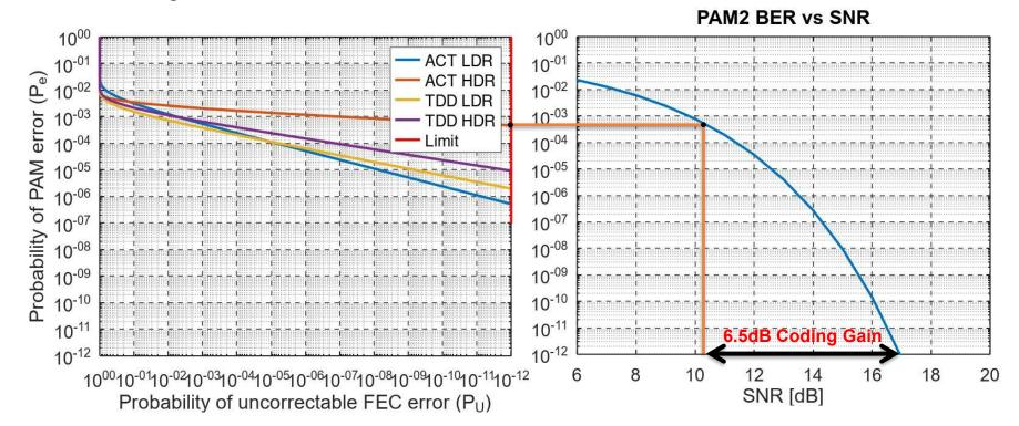
FEC Coding Gain comes from tolerance to higher PAM-symbol error probability
