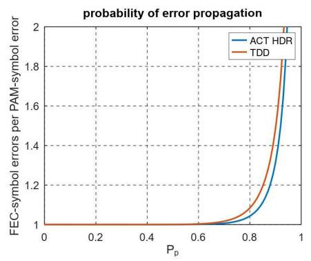
NOTE: The difference between the ACT and TDD RS-FEC in the plot is because the ACT uses 10-bit FEC-symbols, while TDD uses 8-bit FEC-symbols
