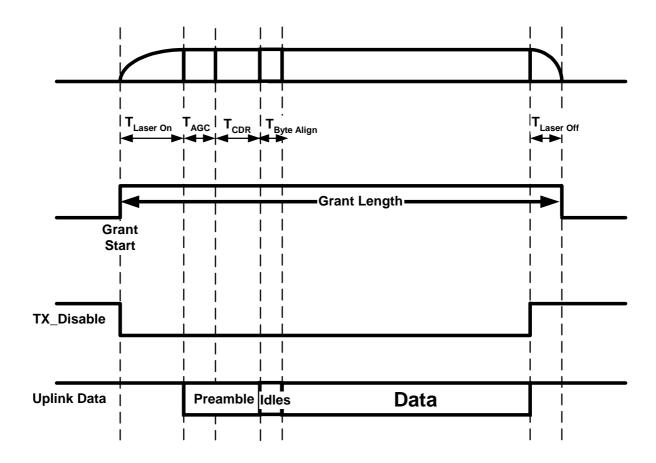
Denote  $T_{laser\_on}$  as the time from the falling edge of the TX\_disable line to the time that the optical power reaches (90%?) of its Average launch power (And opening of the eye diagram to its specified parameters), as presented in the figure above. The data transmitted maybe any valid 8B/10B symbols.
