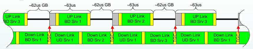
Up Link Guard Band Is Provisioned By The Amount Of Bidirectional Traffic Supported On The Deployed Service Span
