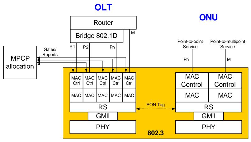
Pi: Point-to-point link to ONUi M: Point-to-multipoint link
