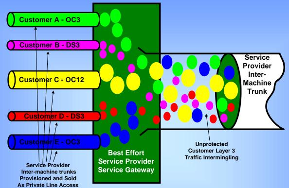
Non-Connection Oriented, Layer 3 service over Layer 3 Infrastructure, Burstable Bandwidth, Low Security, Low to Moderate Reliability, Low to Moderate Availability, Low Data Stability, Self-Autonomous Routing, Low Cost to Customer without Distance Charges (only access distance charges), Low/Negative SP Margins (often this service is subsidized by content services)
