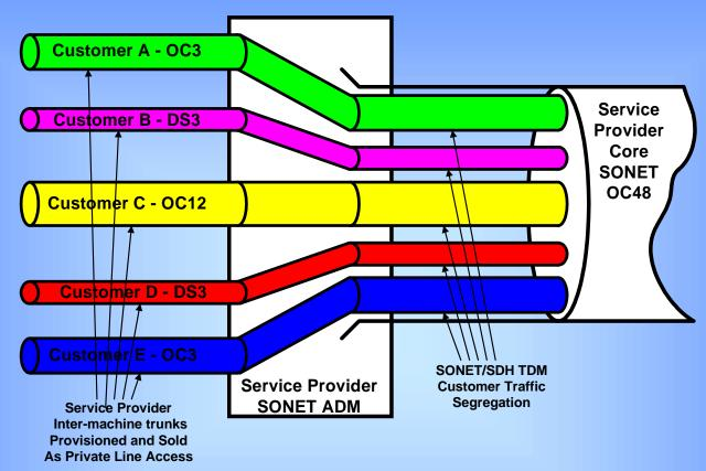
Connection Oriented, Layer 1 Service over Layer 1 Infrastructure, Fixed Bandwidth, High Security, High Reliability, High Availability, High Data Stability, Fixed Routing through Infrastructure, Out of Band Management, High Cost to Customer because of Distance Charges, High Margins to SP
