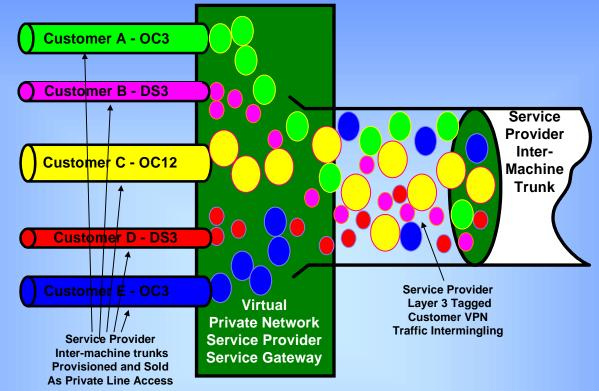
Semi-Connection Oriented, Layer 3 service over Layer 2/3 Infrastructure, Fixed and Burstable Bandwidth, Moderate Security, Moderate to High Reliability, Moderate Availability, Moderate Data Stability, Self-Autonomous Routing, Moderate Cost to Customer without Distance Charges (only access distance charges), Moderate Margins to Service Provider
