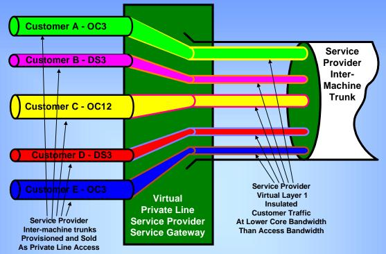
Connection Oriented, Layer 2 service over Virtual Layer 1 Infrastructure, Fixed and Burstable BE Bandwidth, High Security, Moderate to High Reliability, Moderate to High Availability, Moderate to High Data Stability, Implementation Specific Routing Autonomy, Moderate Cost to Customer without Distance Charges (only access distance charges), Moderate SP Margins
