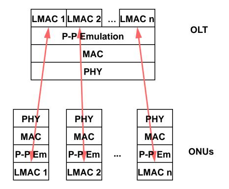
FIGURE 2. MAC model for Point-to-Point LAN Emulation
