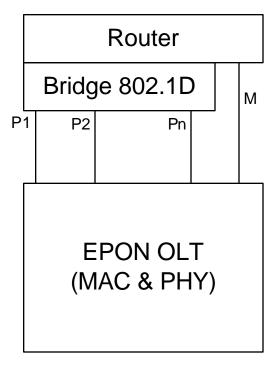
Pi: Point-to-point link to ONUi M: Point-to-multipoint link
