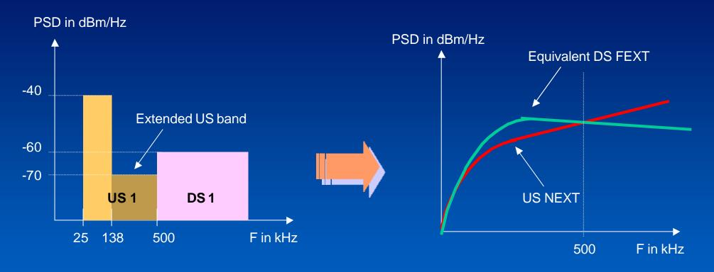
Below 500 kHz, the NEXT induced by US signal transmitted in the DS band remains below the equivalent DS FEXT
