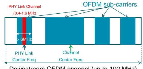
Downstream OFDM channel (up to 192 MHz)
