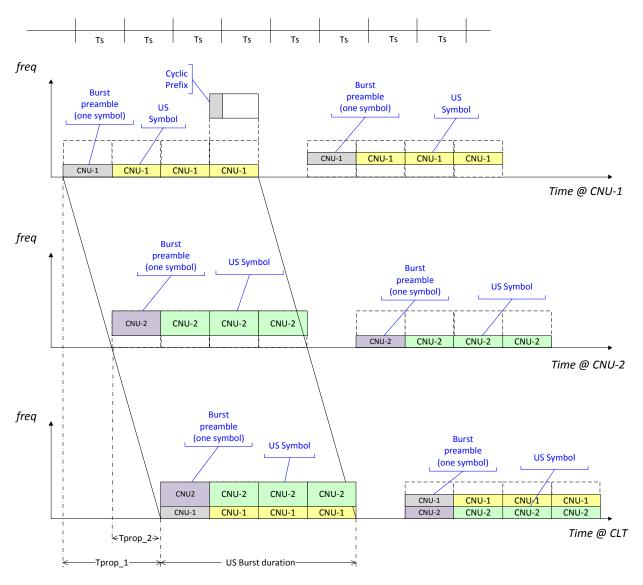
In case of FDD upstream there is a burst transmission consisting in a sequence of upstream symbols
