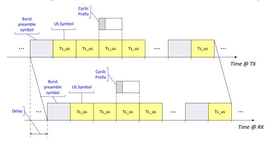
In case of FDD upstream there is a burst transmission consisting in a sequence of US symbols and potentially starting with a burst preamble (of Np\*symbol duration)
