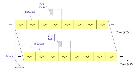
In case of FDD downstream there is a continuous transmission consisting in a sequence of DS symbols
