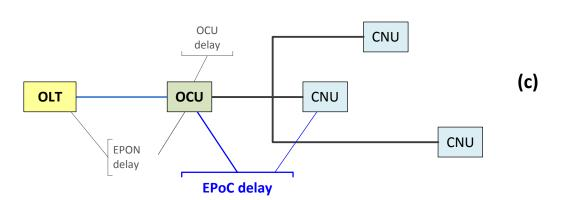
Similarly, the case of EPON with digital fiber can be easily considered adding EPON delay and OCU delay terms.
