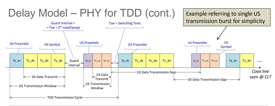
$$TDD \ Transmission \ Cycle = T_{DS\_TXwin} + [\ 2*T_{SW} + 2*max(T_{prop})\ ] + T_{US\_TXwin} \\ = T_{DS\_TXdata} + T_{DS\_TXgap} \\ = T_{US\_TXdata} + T_{US\_TXgap}$$
