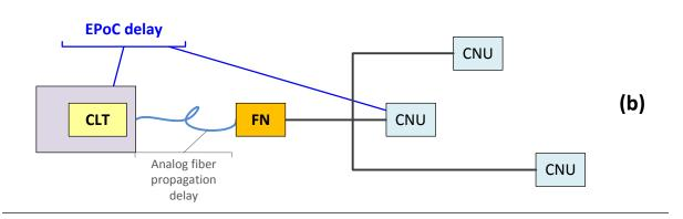
The case of EPoC deployed with analog fiber and CLT in headend can be easily considered adding analog fiber delay as function of the optical fiber length.
