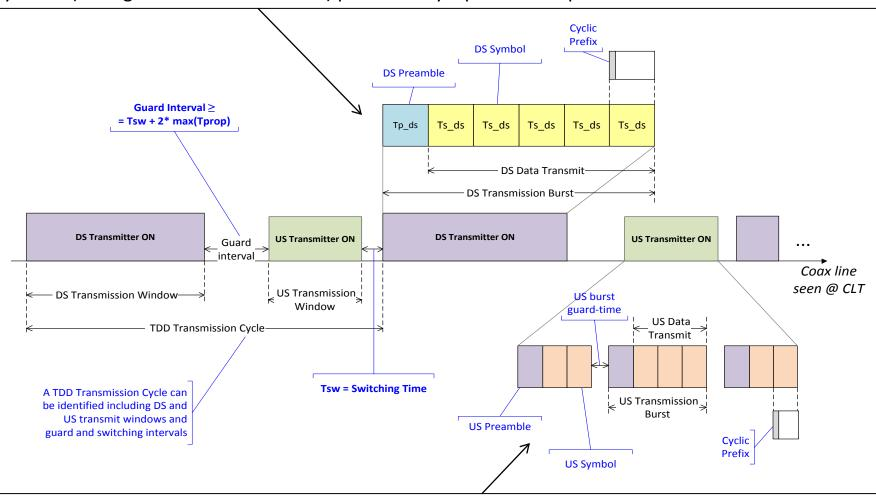
US transmission occurs in the US transmission window and consist in a sequence of US transmit bursts, each of them including data symbols (US data transmit) and preceded by a possible US preamble.
