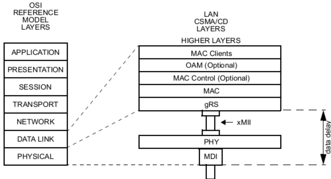
Figure 90-3—Data delay measurement
