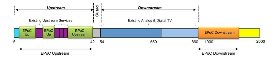
NOTE: This is one illustrative example of spectrum provisioning. There are many other examples including EPoC UP in portion of 1000MHz to 2000MHz region instead in 5 - 42MHz region
