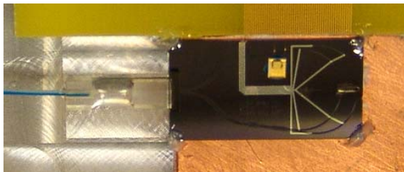
PLC demodulator for 53.5 Gbaud
