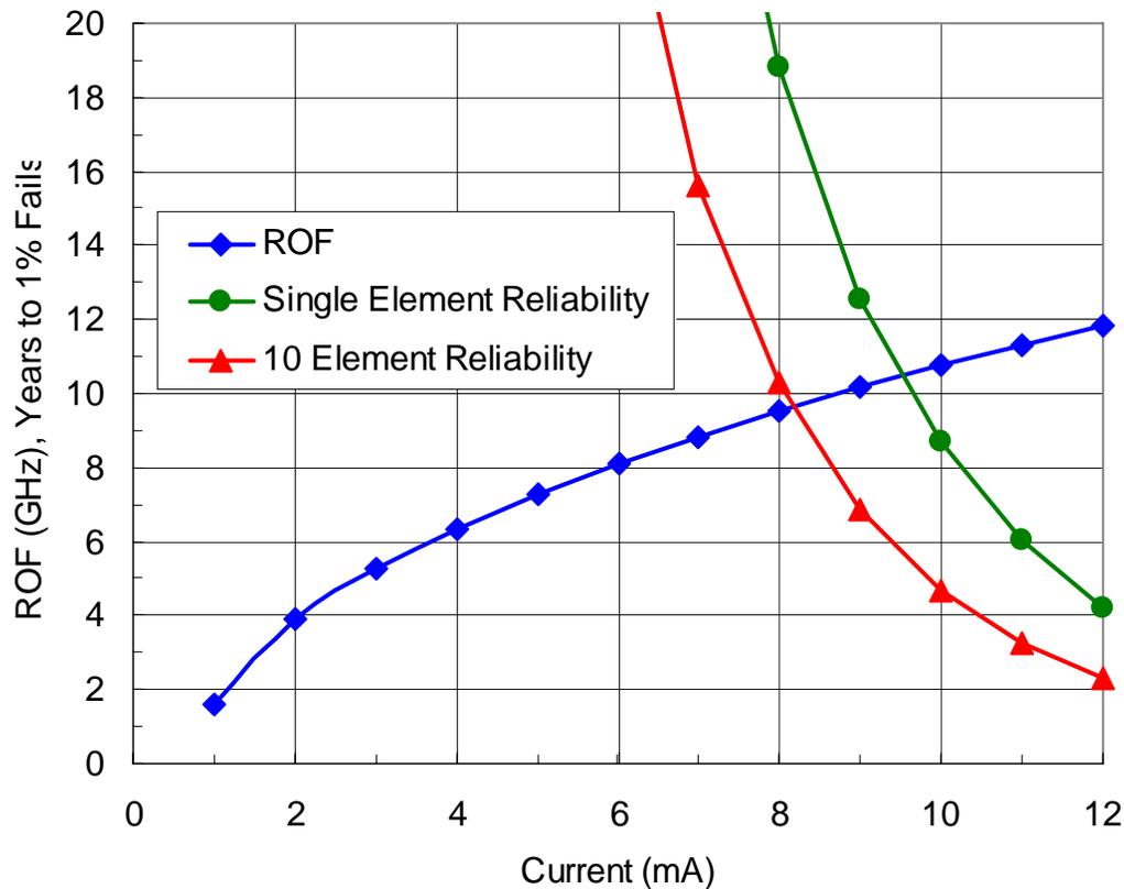
▶ The desire to increase the operating current to increase the speed must be balanced by the reduction in reliability. Data shown for 85C ambient operation
