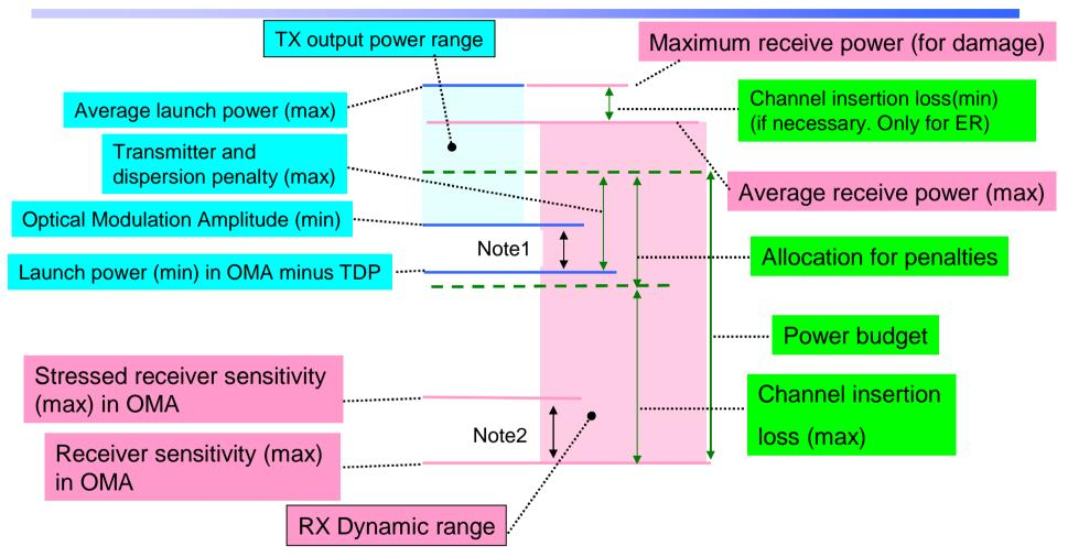
Note1:Even if the TDP < 0.4 dB for ER and <1.0dB for LR, the OMA(min) must exceed this value.
