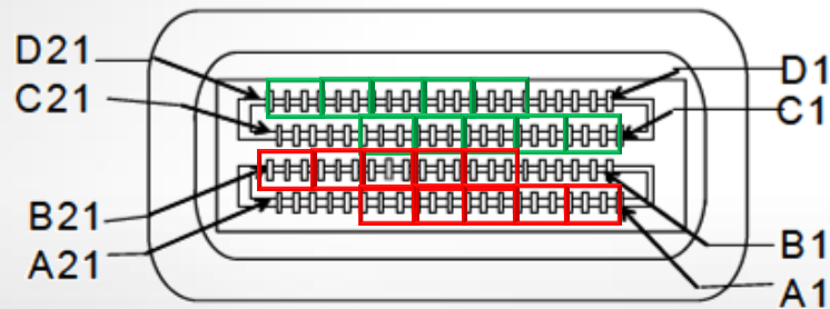
Figure 85-25—Example MDI board receptacle
