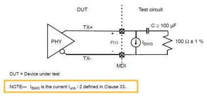
Figure 25–1—Type 2 system time constant test circuit
