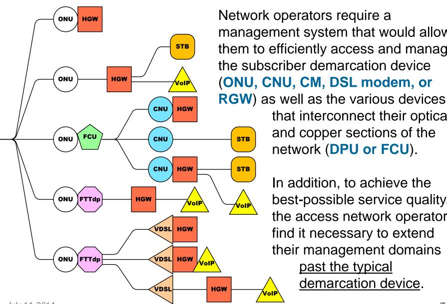
Network operators require a management system that would allow them to efficiently access and manage the subscriber demarcation device (ONU, CNU, CM, DSL modem, or
