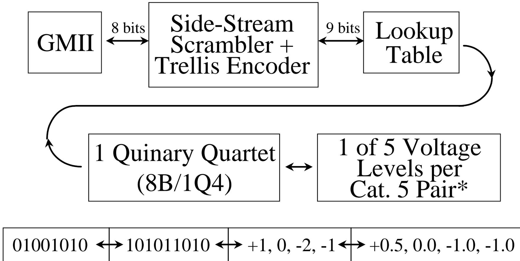
\* Actually 17 voltage levels to reduce emissions by shaping the output
