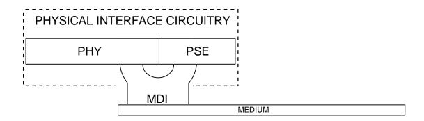
Figure 33--2--DTE Power via MDI Midspan Power Sourcing Equipment (PSE) relationship to the Physical Interface Circuitry and the IEEE 802.3 CSMA/CD LAN model
