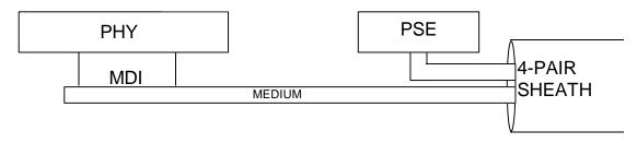
Figure 33--3--DTE Power via MDI Endpoint Power Sourcing Equipment (PSE) relationship to the Physical Interface Circuitry and the IEEE 802.3 CSMA/CD LAN model
