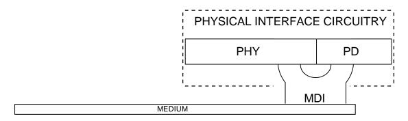
Figure 33--1--DTE Power via MDI Powered Device (PD) relationship to the Physical Interface Circuitry and the IEEE 802.3 CSMA/CD LAN model
