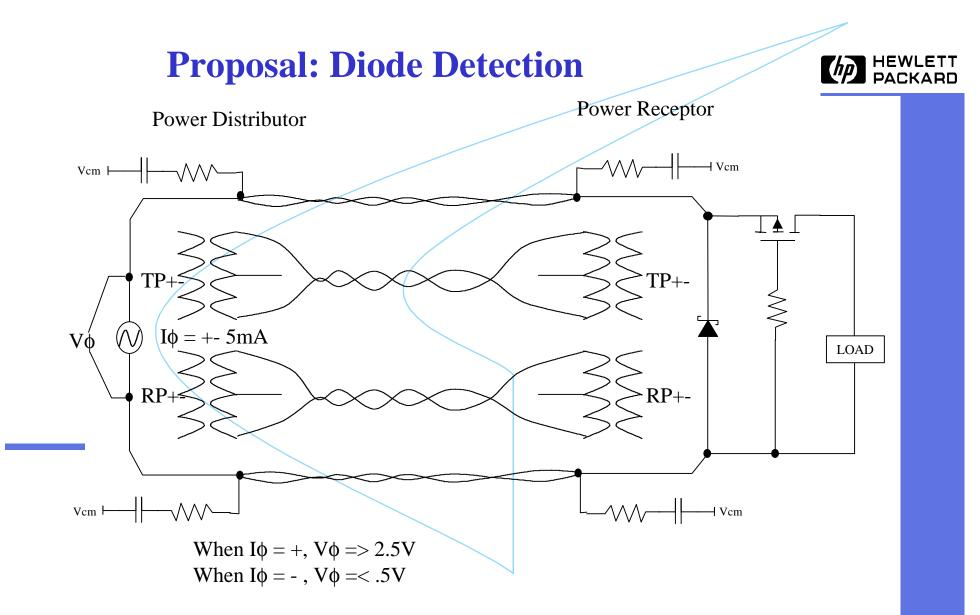
**Invent!** Therefore, comparators set to  $\pm 1.5$  volts will detect proper mode with 0,1,0,-1.. IEEE 802.3ae Interim - Dallas - Jan 2000
