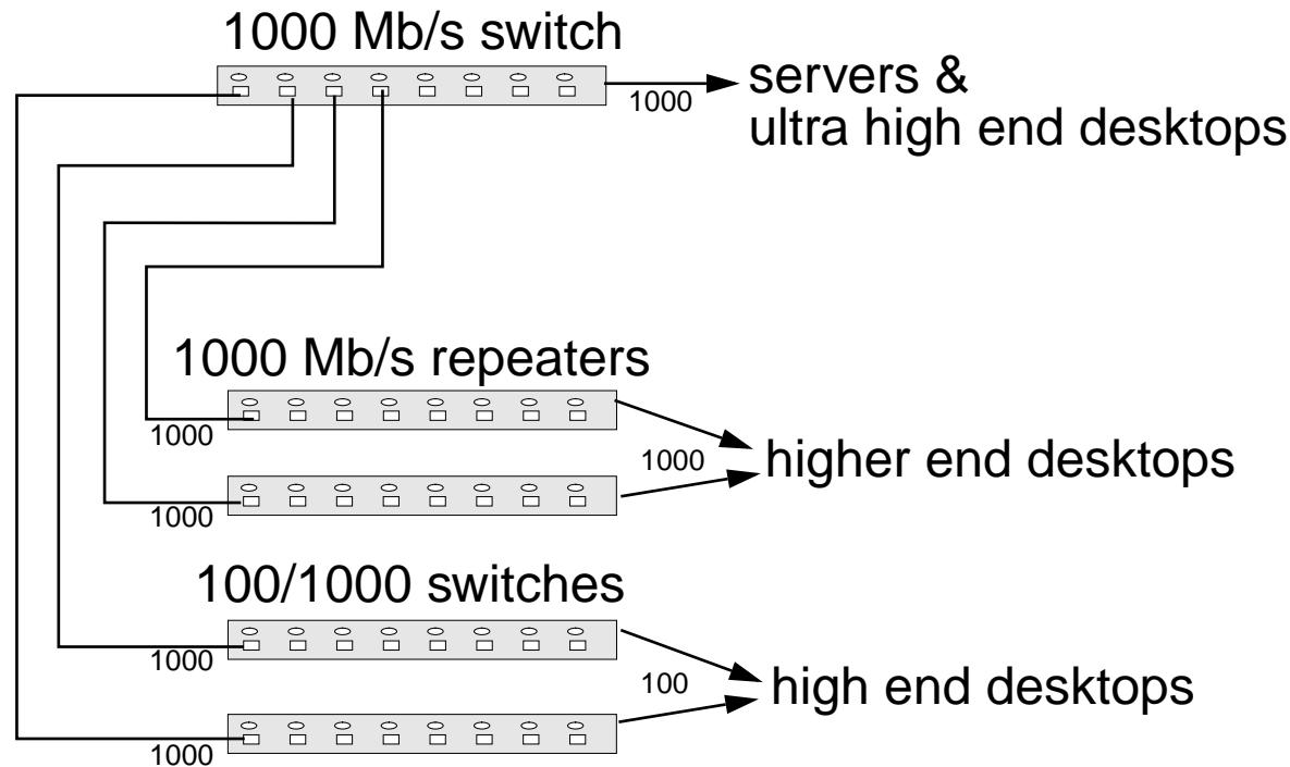
CSMA/CD used in single repeater collision domains
