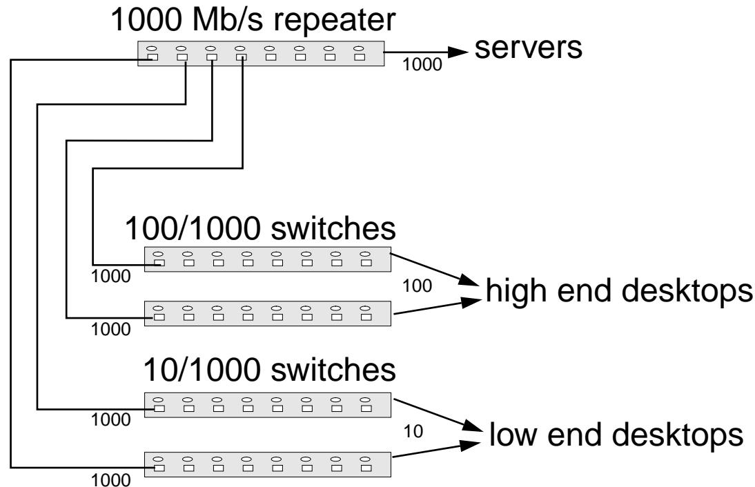
CSMA/CD used in a single repeater collision domain
