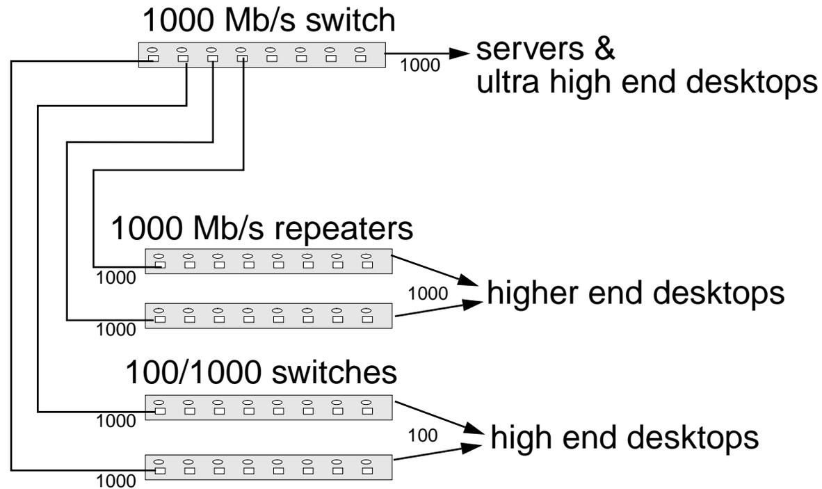
CSMA/CD used in single repeater collision domains
