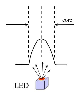
LEDs spray light in a wide pattern into the core, illuminating many modes of propagation.
