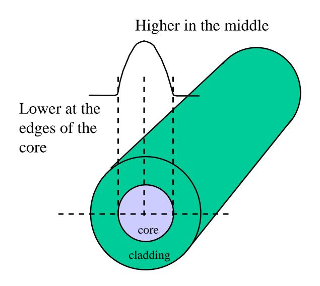
This core profile supports many modes optical of propagation
