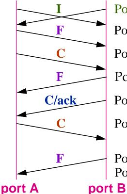
Ports active Port A starts Power\_Off procedure Port A Link\_Configuration w/Offline Port B recognizes Port A Link\_Startup Port B LCAck of Port A offline Port A signals Offline for a minimum time
