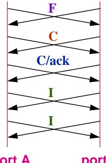
Port A power on, Port B power on Ports exchange Link\_Configuration data Ports exchange Link\_Configuration Acks
