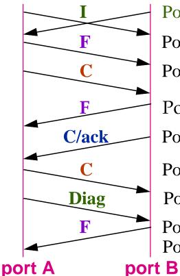
Ports active Port A starts Power\_Off procedure Port A Link\_Configuration w/Offline Port B recognizes Port A Link\_Startup Port B LCAck of Port A offline Port A signals Offline for a minimum time Port A signals Offline for a minimum time Port A starts diagnostics; Port B awaits Link\_Startup from Port A
