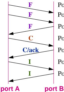
Port A power on, Port B power off Port B power still off Port B power on Port A Link\_Configuration to Port B Port B Link\_Configuration, Ack Port A Port A ready Port B ready
