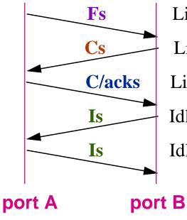
Link\_Not\_Available Link\_Configuration Link\_Configuration w/Ack Idle Idle
