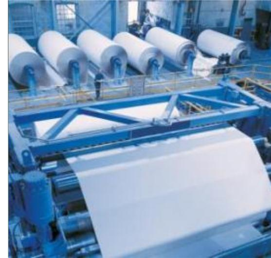
Printing machine: Large number of synchronized axles
