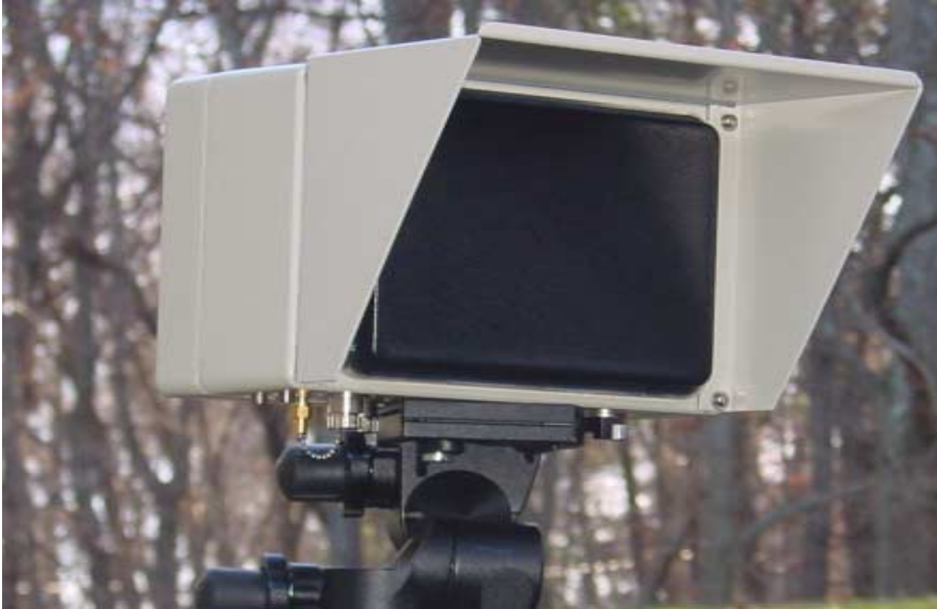
Quarter Mile Solution with Patch Array Antenna
