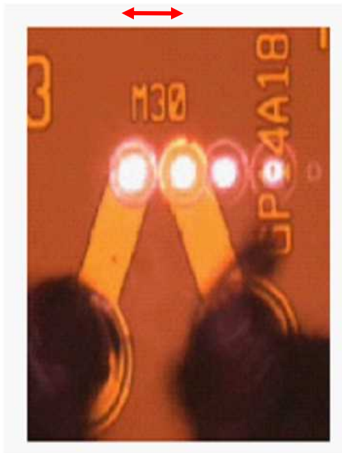
Photograph of monolithic two wavelength VCSELs
