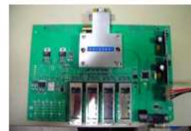
Figure 7b: Optical backplane connector on line card
